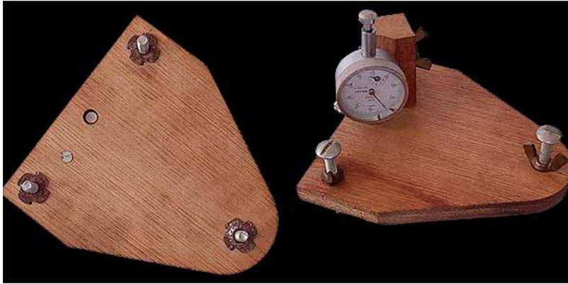
I also made this bed-resting base but don't use it very often. Simple to make using 1/4" screws, wing nuts and 'T' nuts so the height is adjustable.
